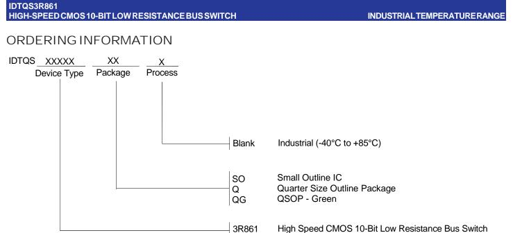
High Speed CMOS 10-Bit Low Resistance Bus Switch with Flow-Through Pinout
